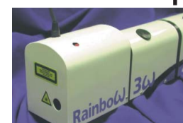
RAINBOW – OPO laser 340–475 nm ~ 5 mJ 410–680 & 720–1 100 nm ~ 55 mJ 680–970 & 1 200–2 000 nm ~ 80 mJ
